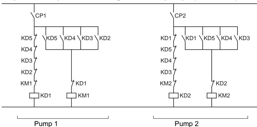
For pumps 3 to 5, same diagrams, incrementing the indices (KDx, KMx, CPx).
