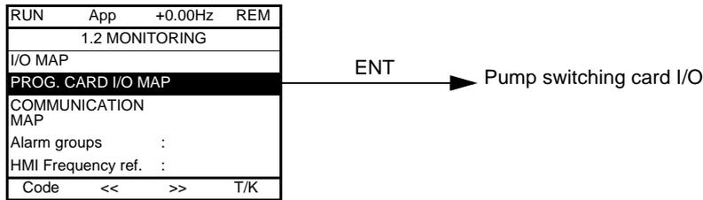
The presence of the pumps can be checked via the state of the logic inputs on the pump switching card.
