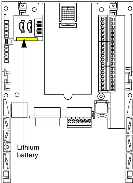
When installing the pump switching card in the drive, make sure that this battery is present. It takes the form of a rectangular block clipped onto the non-volatile RAM (see schematic opposite).
