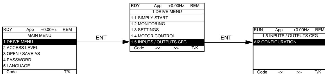
Configure AI2 according to the pressure sensor being used (Example: 4 - 20 mA)
