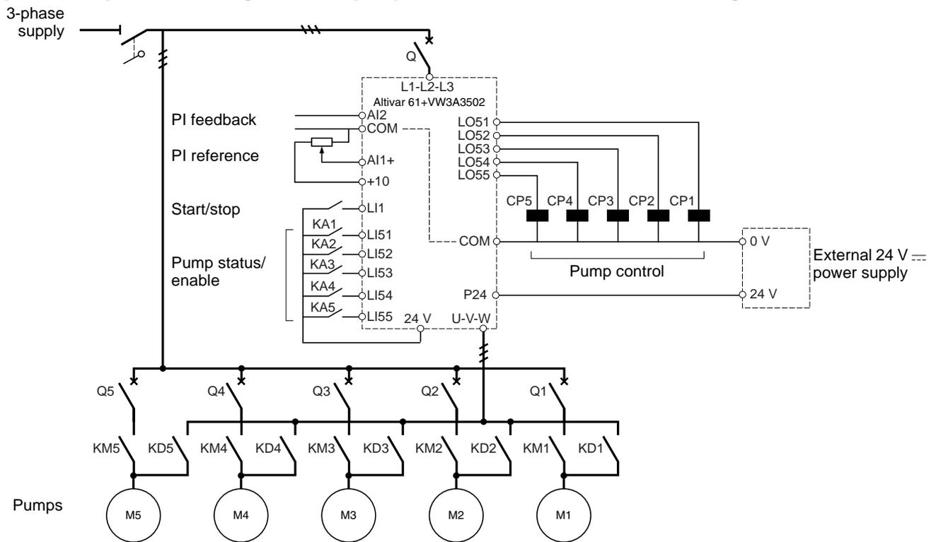
Each pump is controlled by a logic output.
