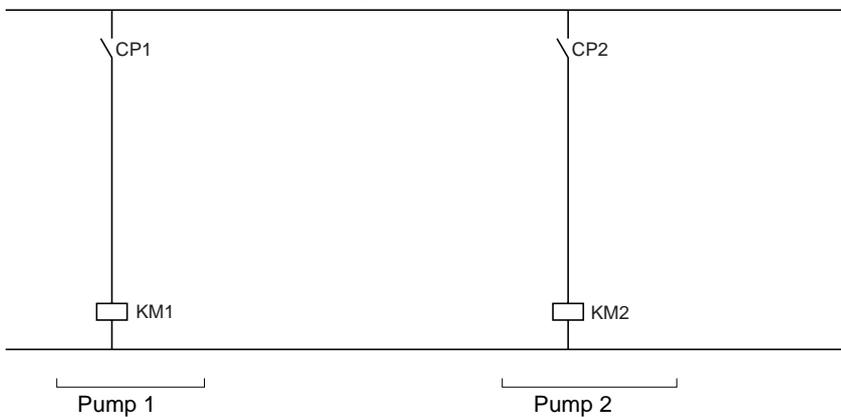
For pumps 3 to 5, same diagrams, incrementing the indices (KMx, CPx).
