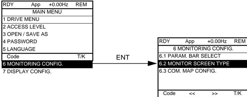
**[6.2. MONITOR SCREEN TYPE]:** Selection of parameters displayed in the centre of the screen and the display mode (digital values or bar graph format).
