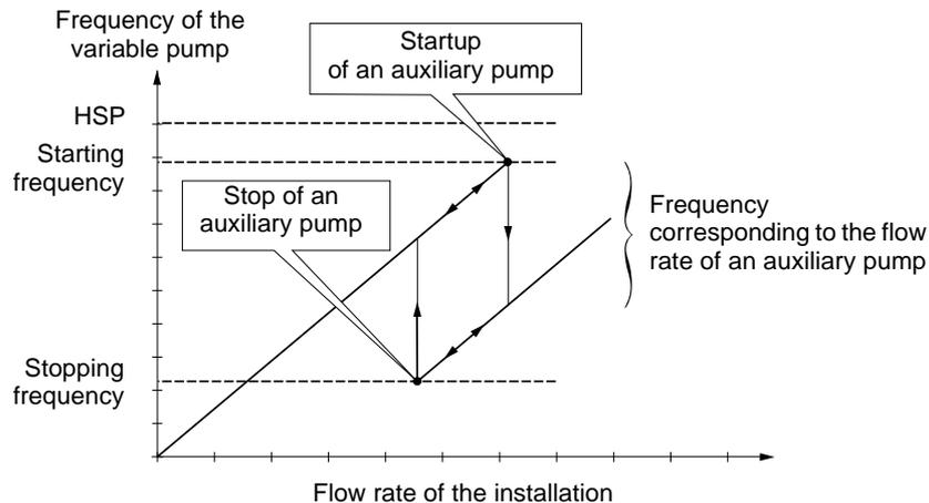
When the frequency exceeds the starting threshold (**[FrqAuxPumpOn] (O12)** parameter), a time delay (**[Pump Delay On] (O03)** parameter) is started to avoid the effects of transient flow fluctuations. If after this time delay, the frequency remains higher than the starting threshold, another pump is started. When the start command is sent, a time delay (**[Acc Aux Pump] (O06)** parameter) is started to allow the pump to reach its nominal speed before starting another pump (avoids oscillation).
